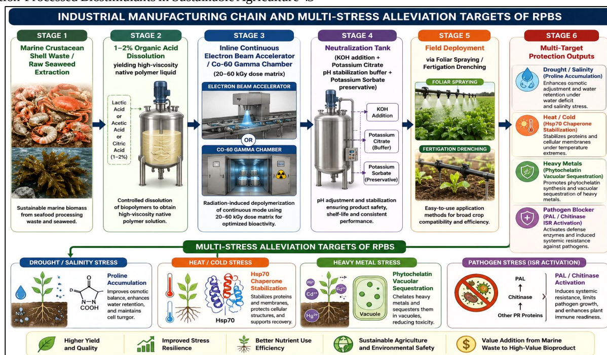
Fig. 2 : Industrial manufacturing pathway and multi-stress protection targets of radiation-processed biostimulants. The diagram tracks the sequence from raw marine byproduct preprocessing to continuous inline radiolytic chain scission, formulation stabilization and subsequent activation of tolerance mechanisms against abiotic and biotic stresses (Patil and Joshi, 2024; Zhou and Sharma, 2025).
